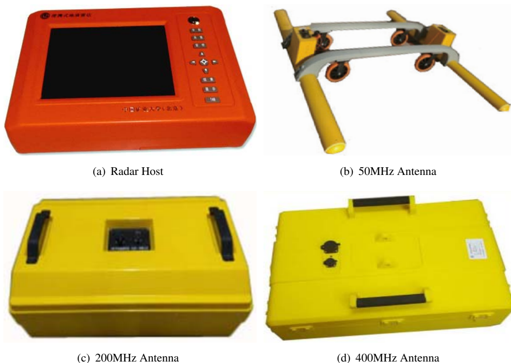
Figure 2. Employed GPR tools with a host and three antennas with 50 MHz, 200 MHz and 400 MHz, respectively.
