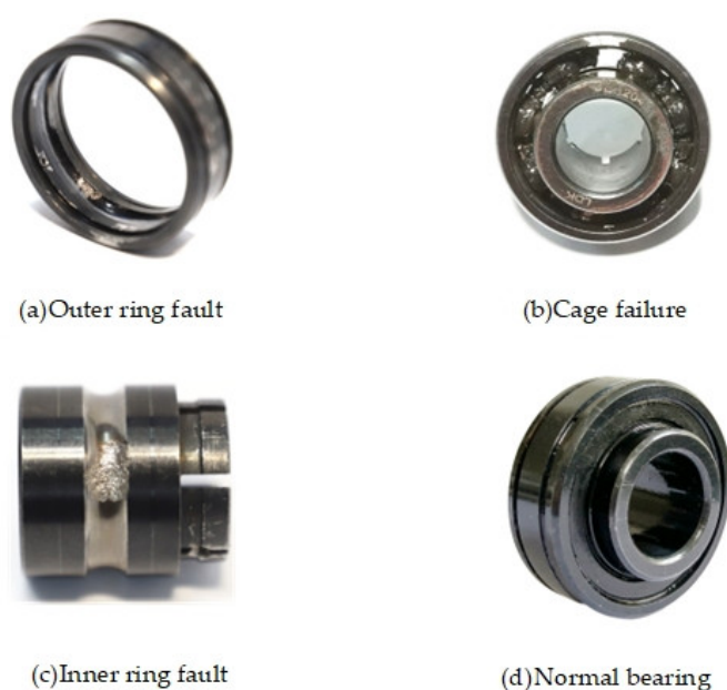
Figure 8. Bearing failure pattern.
