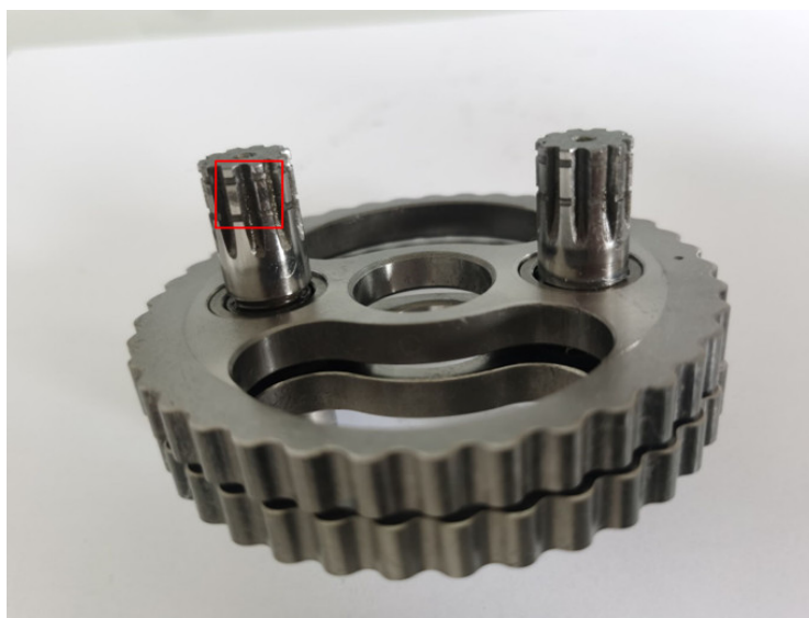
Figure 12. The crankshaft is worn.
