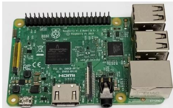
Figure 3. Raspberry Pi 3B.
