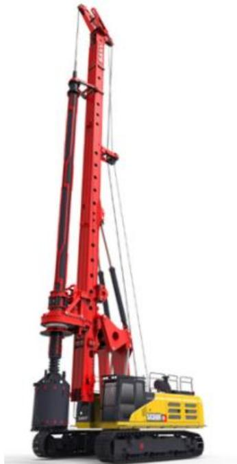
*Figura 4-45 SR150C Perforadora Giratoria (SANY, 2020)*
