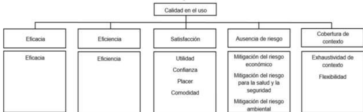
Figura 7. Modelo de Calidad en Uso. Adaptado de “Systems and software engineering -- Systems and software Quality Requirements and Evaluation (SQuaRE) -- System and software quality models”, ISO/IEC 25010, 2011.
