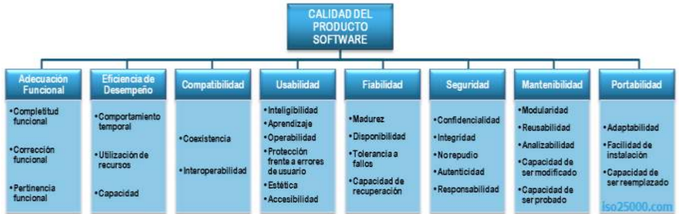
Figura 4. Características de calidad. Adaptado de “SQuaRE (System and Software Quality Requirements and Evaluation)”, ISO/IEC 25000, 2014.
