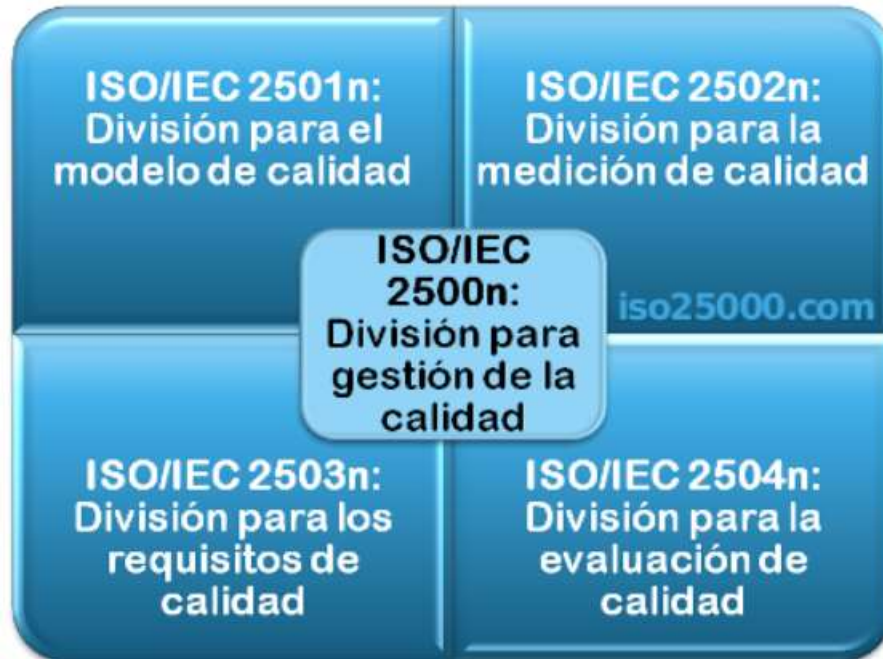
Figura 3. Divisiones ISO/IEC 25000. Adaptado de “ SQuaRE (System and Software Quality Requirements and Evaluation) ”, ISO/IEC 25000, 2014.
