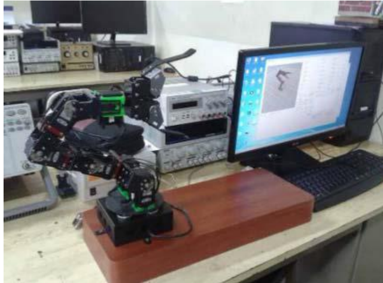
Figura 1.3: Proyecto “BRACON: Control system for a robotic arm with 6 degrees of freedom for education systems” – Ecuador. 19
