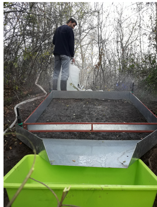
Figure 3. The rainfall simulator during filed operation
