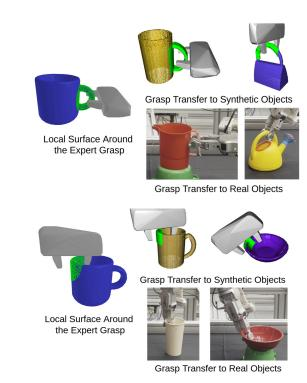
Fig. 1. Example experiments of grasp transfer to various objects. Utilizing implicit representations of local surfaces, grasps are transferred to novel objects by identifying local surfaces that are geometrically similar to those surrounding the expert grasps.
