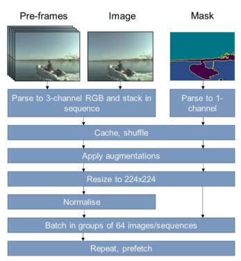
Fig. 11. The data pipeline for training data.
