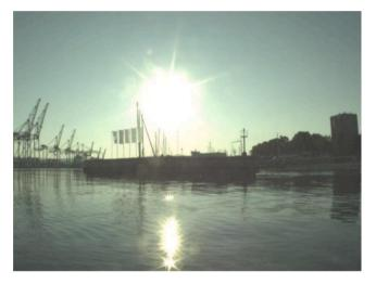
**Fig. 2.** Example of image captured on-board a USV. In this example both strong glare and obstacle reflections in the water make the scene challenging for computer interpretation Bovcon et al. (2022).
