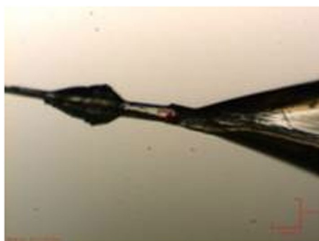
Fig. 2 A crystal of RNase A mounted for data collection at Diamond
