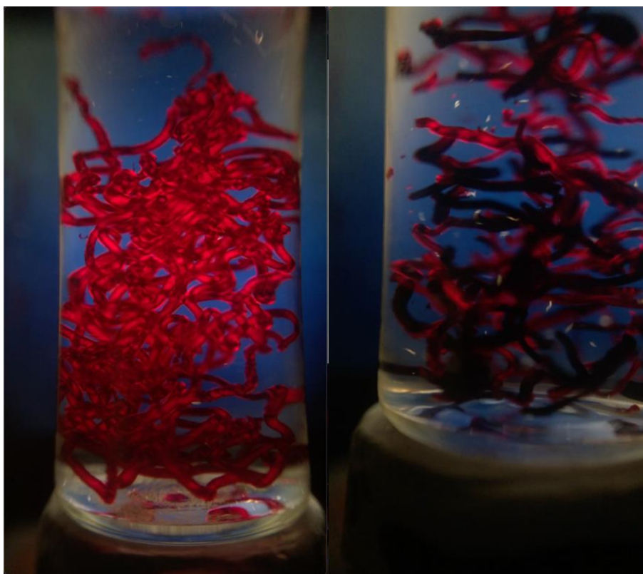
Figure 39- Image of PBI-I noodles before (L) and after (R) illumination with a Xe lamp. The bright sections in the picture before illumination demonstrate an element of alignment in the noodles as a result of shear forces. The image taken after the illumination appears to have entire noodles that appear dark which suggests they have lost alignment upon illumination.
