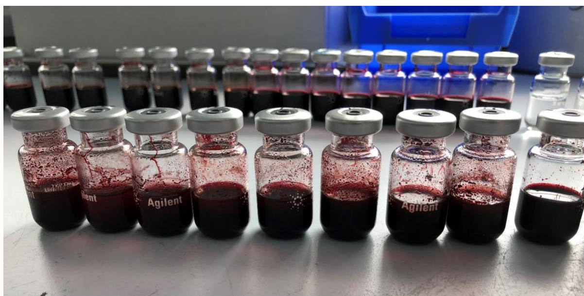
Figure 13- (Top) Image of the purging of many PBI samples at once, before being transferred to the solar simulator. (Bottom) Image of the sample preparation of PBI dispersions. Each sample was 5 mg/mL PBI, with 20 (v/v%) methanol and contained platinum nanoparticles (1 wt.%). The samples in picture were each at a different pH and therefore display different levels of aggregation.
