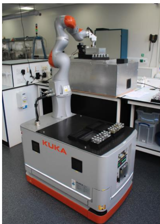
Figure 5- An image of the autonomous robot performing photocatalysis experiments. Taken from literature with permission. 63
