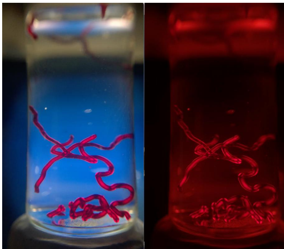
Figure 38- Image of crossed noodles, will probably just go with one of these. Crossed sections appear dark due to additional effect of polarising light due to birefringence. Red filter used to confirm difference due to birefringence and not absorbance in visible region from PBI noodles.
