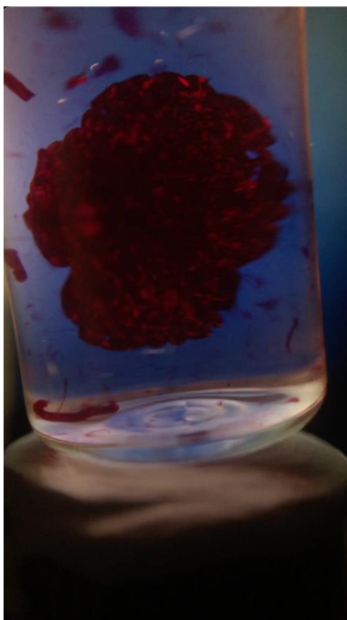
Figure 41- Unaligned clump of PBI-I noodles which was used for initial photocatalysis testing to compare with aligned noodles. Clump was formed due to noodles dissolving on top of one another in water, before the addition of concentrated \text{Ca}^{2+} locked in the structure. This sample was then illuminated for 3 hours before headspace gas analysis.
