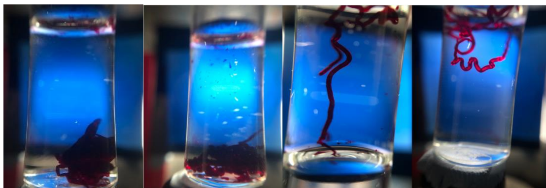
Figure 37- Images of PBI-I noodles on 4 sequential days with slight differences in pH and therefore alignment. First picture pH= 6.32, second picture pH= 6.66, third picture pH= 5.95, and the fourth picture pH= 6.12. The pH of the PBI-I solution was adjusted using low concentrations of HCl or NaOH with stirring and left overnight to sit without stirring. Brighter sections in image 4 illustrate aligned noodles.
