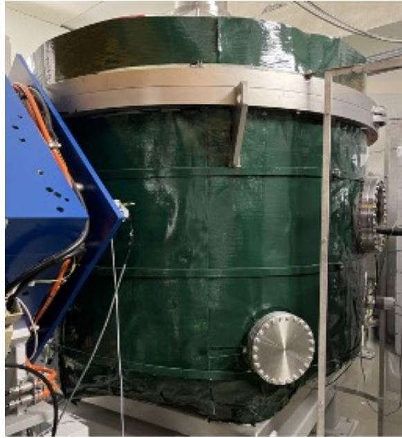
Fig. 3.8 A picture of the electrical dipole which is located behind the quadrupole triplet.
