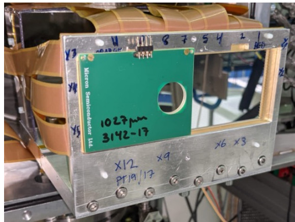
Fig. 3.12 Photograph of the Punch-through detector, also known as the Veto detector, installed just behind the DSSD at MARA's focal plane (only one part appears in the photograph).
