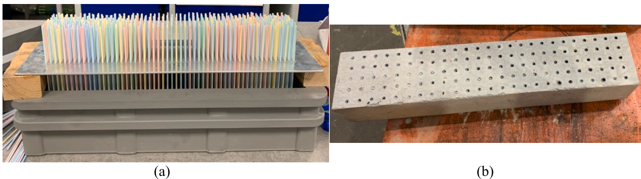
Fig. 2. Stages of CRP preparation: (a) plastic tubes held in place using a timber base and steel plate at top of the mould; and (b) final ground sample prior to testing.
