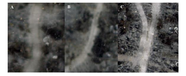
**Figure 2.6**: Rhizotron scanning surface experiment comparing imaging quality for **A**) 4 mm thick, low iron, reinforced glass, **B**) acrylic - 5 mm thick and **C**) acrylic - 2 mm thick, scanned at 1,600 dpi.
