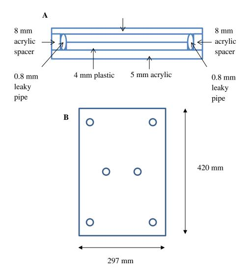
**Figure 2.2**: Schematic diagram of new minirhizotron design B A) Top view and B) Front view (circles indicate screws).
