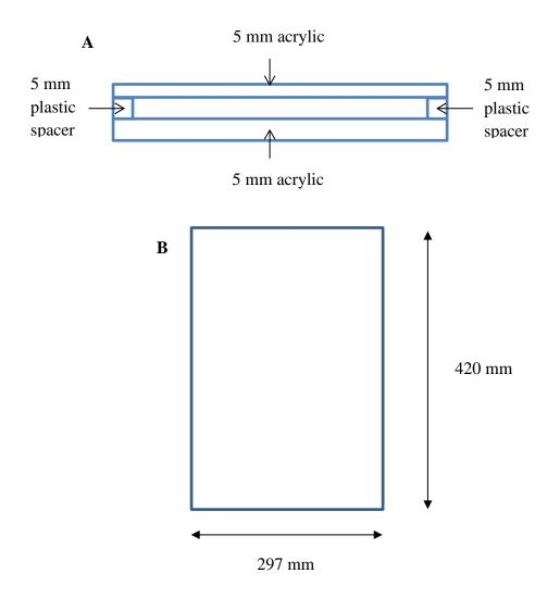
**Figure 2.1**: Schematic diagram of the starting minirhizotron design **A**) Top view and **B**) Front view.
