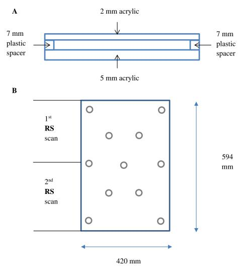
Figure 6.1: Schematic diagram of the proposed A2 sized **RS** unit **A**) Top view and **B**) Front view.
