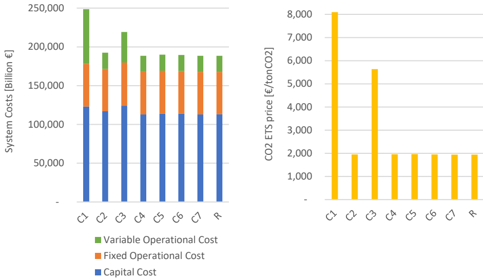
Figure 48, Comparison of system costs (left) and CO2 price (right) in 2050 with the reference case (i.e. R). Eight different cases are used to explore the flexibility enhancements in IESA-Opt. By only neglecting shedding flexibility options, system costs and emission prices increase drastically.
