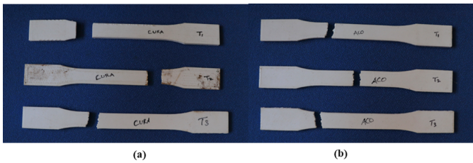
Fig. 12. Validation of strength printed using G-codes generated by (a) Cura (b) proposed algorithm after the tensile test
