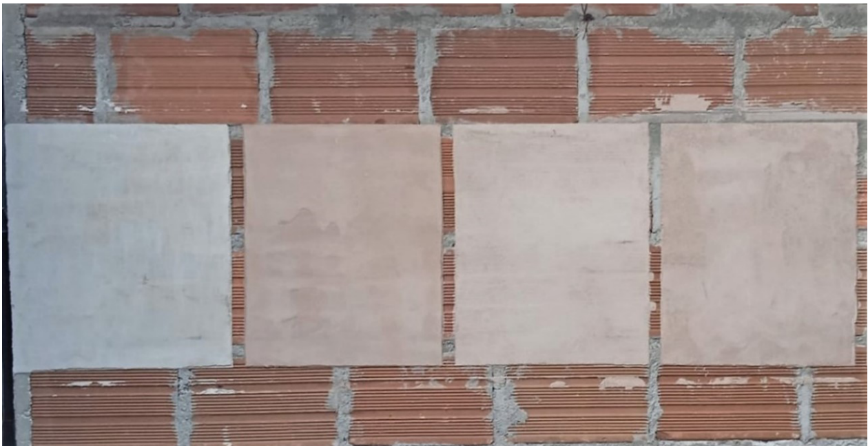
FIGURE 10. Applied mixes, photo at day 60 (from left to right: AC1, A4, A7, A9).
