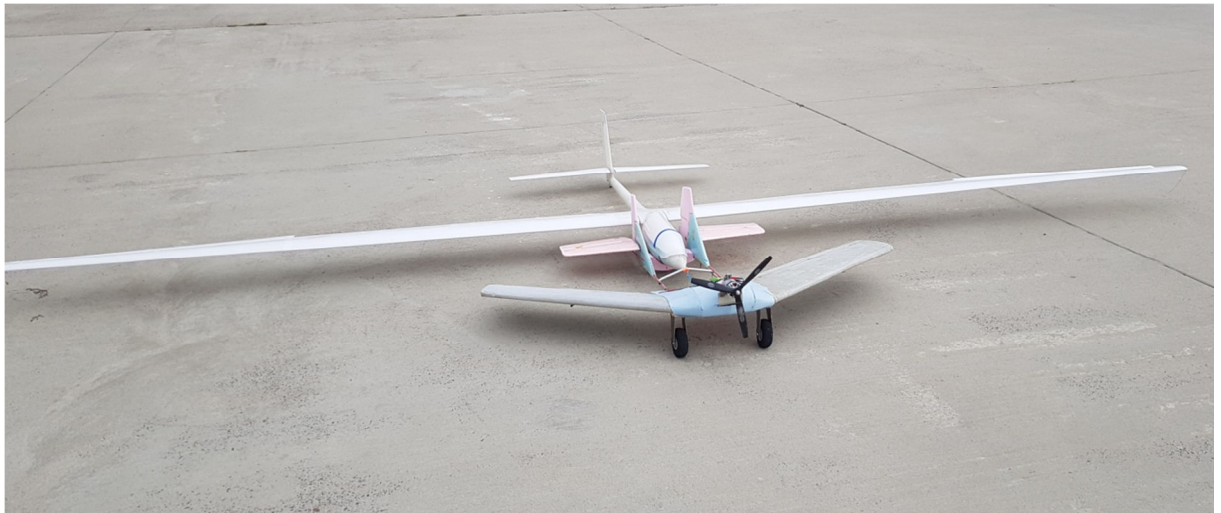
8. Model of the glider and UAV-tug unit - version 2 with lowered engine turret and landing gear with rear support point. Source: T. Muszyński archive
