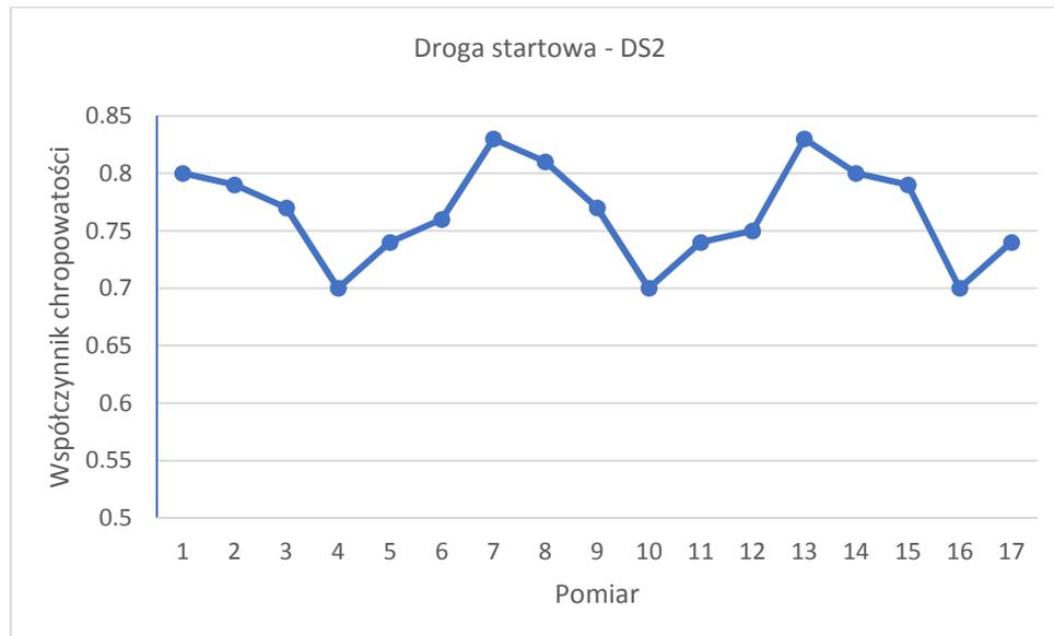
7. The course of variation of the friction coefficient determined for the surface of the runway marked DS2 at the speed of 95 km/h and with a water film
