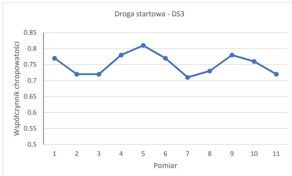
8. The course of variation of the friction coefficient determined for the surface of the runway marked DS3 at the speed of 95 km/h and with a water film
