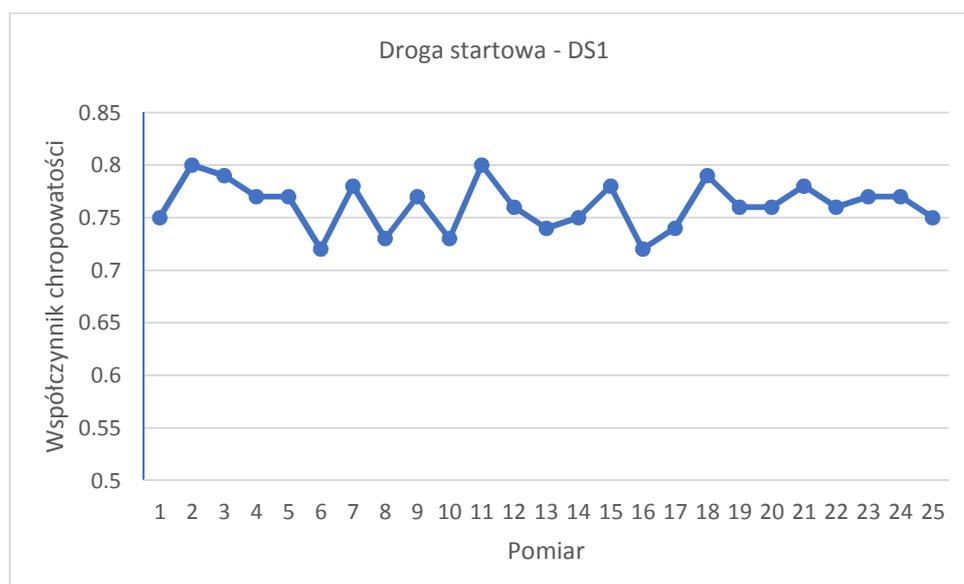
6. The course of variation of the friction coefficient determined for the surface of the runway marked DS1 at a speed of 95 km/h and with a water film
