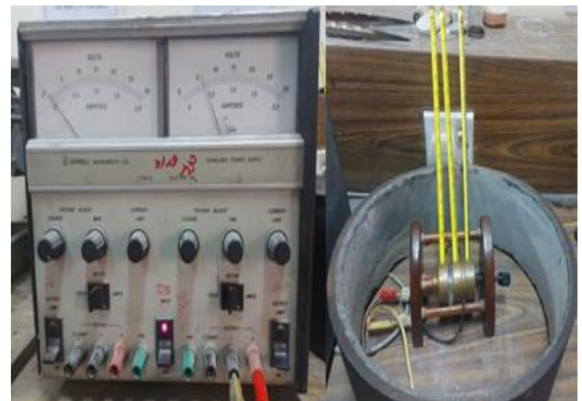
Figure 2. Lee disc apparatus used to measure thermal conductivity
