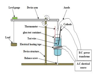
Figure 3. Illustrated a diagram of the static stress corrosion cracking device parts that designed and manufactured locally according to the American Standard (ASTM G10 $\mathcal{E}$  – 97) [15].
