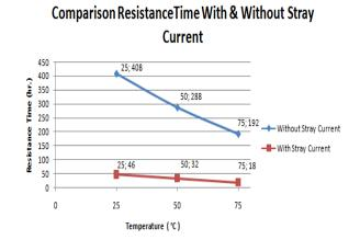
**Figure 4.** A comparison between the durability duration of aluminum electrical wires in the existence and absence of stray currents under different test conditions.
