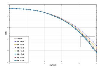
Figure 4. (a) BER performance Comparison of PC OFDM-DCSK for different Clipping Ratio values, N=256 and  $\beta$ =125.
