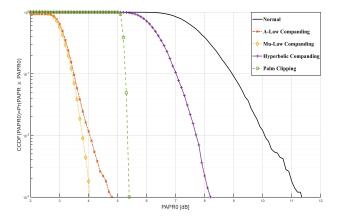
Figure 6. CCDF PAPR performance Comparison for all the tried technique, N=512 and  $\beta$ =125.
