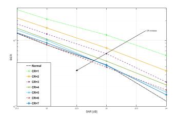
**Figure 4. (b)** BER performance Comparison of PC OFDM-DCSK for different Clipping Ratio values, N=256.
