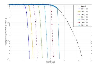
Figure 3. The CCDF of PC OFDM-DCSK for various Clipping Ratio Values, N=256 and  $\beta$ =125.
