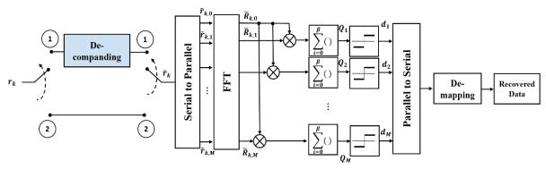
Figure 2. OFDM-DCSK receiver scheme.
