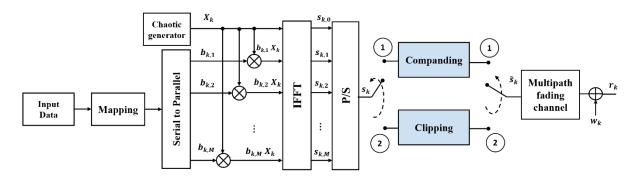
Figure1. OFDM-DCSK transmitter scheme.
