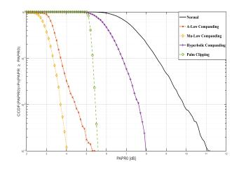
Figure 5. The CCDF PAPR performance Comparison for all the tried techniques, N=256 and  $\beta$ =125.
