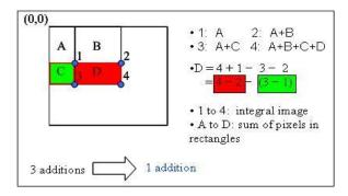
Figure 2. Calculation of integral image
