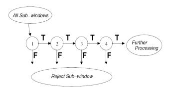
Figure 5. Classifier Cascade Process
