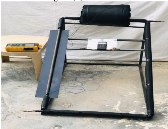
Figure 2. Photo of the thermo syphon device.
