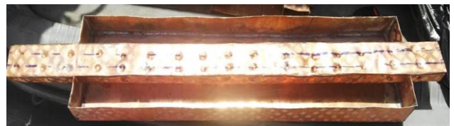
Figure 13. The granular duct
