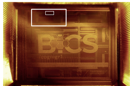
Figure 1: Photograph of the realised die. The small white rectangle indicates the area covered by the synaptic normalisation block, while the larger rectangle encompasses the peripheral supporting circuitry too.
