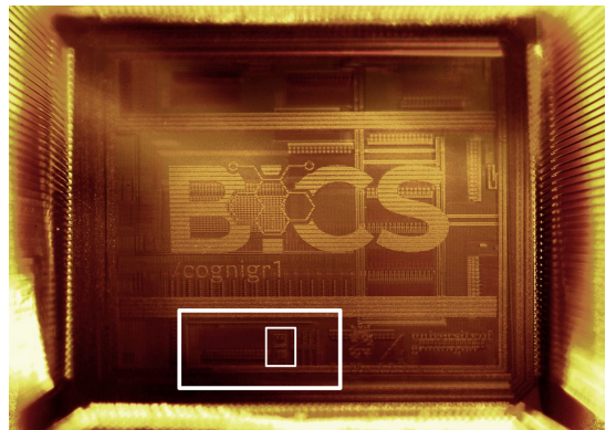
Fig. 1. Photograph of the realised “Cognigr1” ASIC. Within the small white rectangle are the analog synapses and competitive hWTA neuron circuits, while the larger white rectangle includes the on-chip DAC and supporting I/O circuitry.
