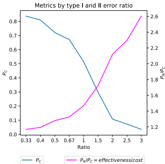
Fig. 6 Performance metrics as a function of the type I and II weighting ratio
