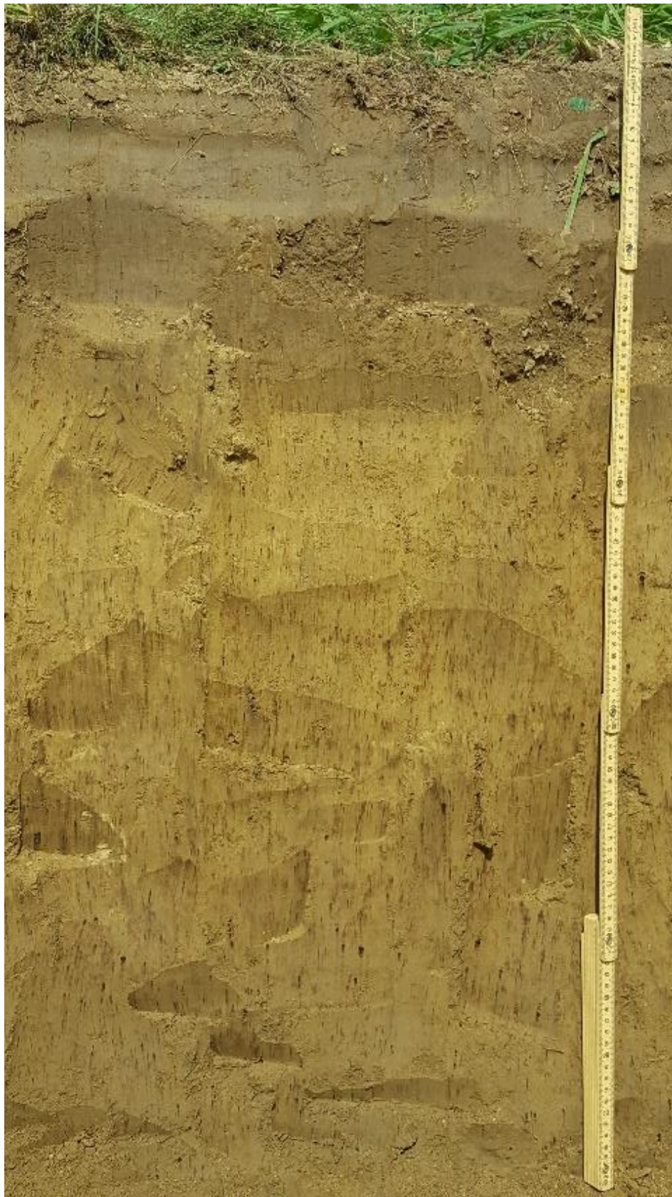
Figure S1.14: Soil profile of the Haplic Luvisol in the DOK experiment. The blackish-brown smears, which are the result of working the profile with a spade, show iron-manganese concretions. See also Figure S1.13 . Photo: Markus Steffens.
