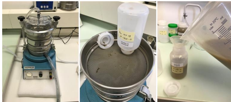
Figure S1.11: Wet-sieving of the mineral fraction after separation of POM fractions.
