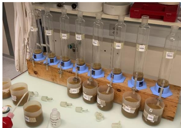
Figure S1.12: Particle size fractionation of the mineral fraction <20 \mu\text{m} via sedimentation.
