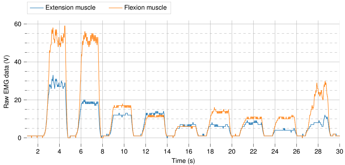
(a) Raw EMG signal from S2 while sitting during rest. Each level is activated for 2 seconds followed by 1 second rest starting with from -4 (flexion) to 4 (extension).
