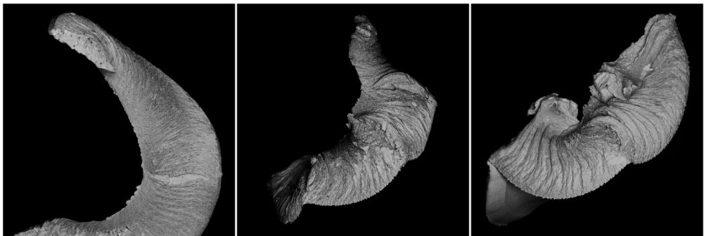
Figure 5.2: Chips from Face Turning 1 (left), 2 (middle), 3 (right).
