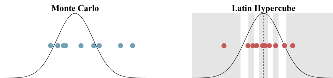
Figure 8. Monte Carlo and Latin Hypercube simulations in one dimension, with N=10 . Black lines show the probability distribution. For the Latin Hypercube simulations, the bins with equal probability are indicated by the filled areas.
