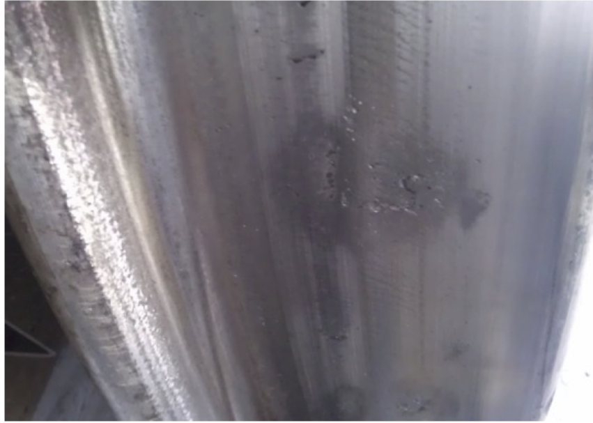
Figure 6: Thermal facets with local crack formation on a railway wheel. Note the different orientations of the thermal cracks and the RCF cracks.
