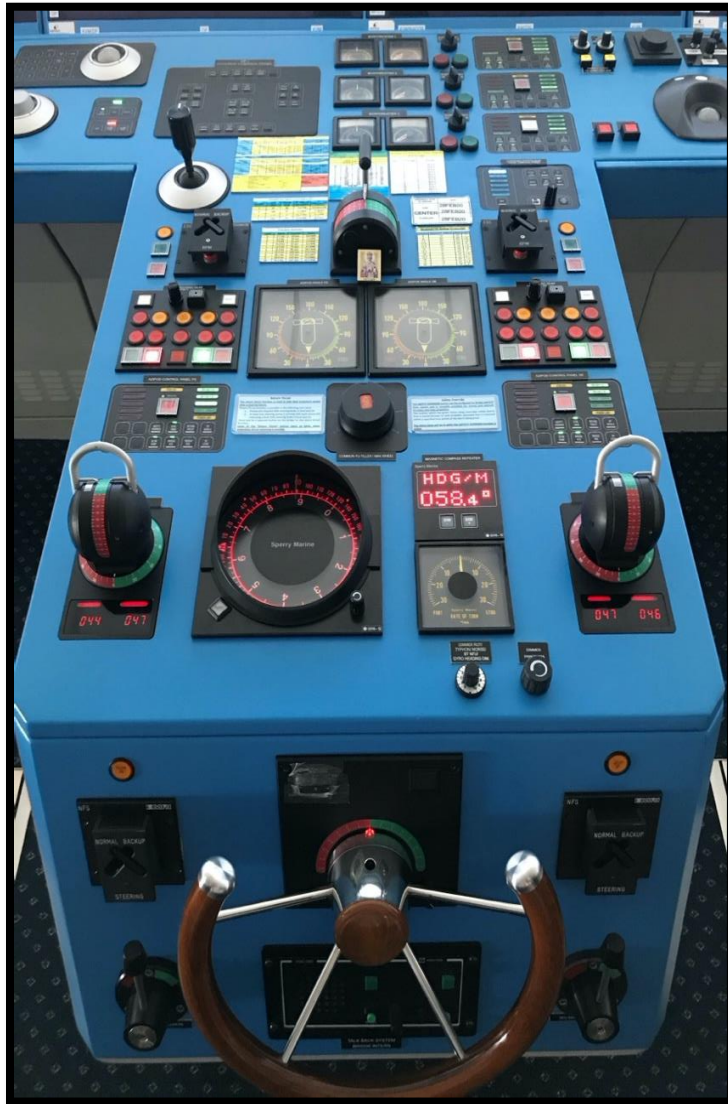
FIGURE 3-3: BRIDGE CONSOLE (SOURCE: OWN ELABORATION)
