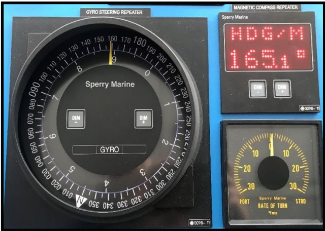
FIGURE 4-2: GYRO AND MAGNETIC COMPASS AND RATE OF TURN INDICATOR (SOURCE: OWN ELABORATION)
