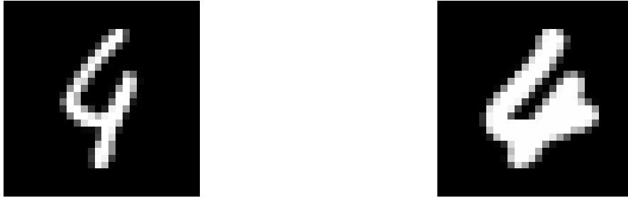
Figure 4.1: Images triggering deviated behaviors between LeNet-4 and its quantized model. The ground truth labels of both images are “4” and both of them are correctly classified as “4” by the original model. However, the quantized model classifies them as “9” and “6” respectively.
