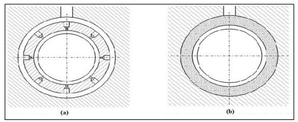
Figure 3: Aerostatic Thrust Bearing (a) with a simple orifice (b) with a porous layer [111]
