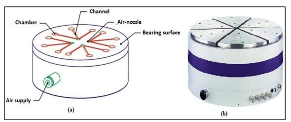
Figure 1: Aerostatic Journal Bearing (a) Schematic View (b) Original View [79]
