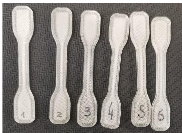
Figure 7. Tensile test specimens printed at 240 °C with a printing speed of 40 mm/s.
