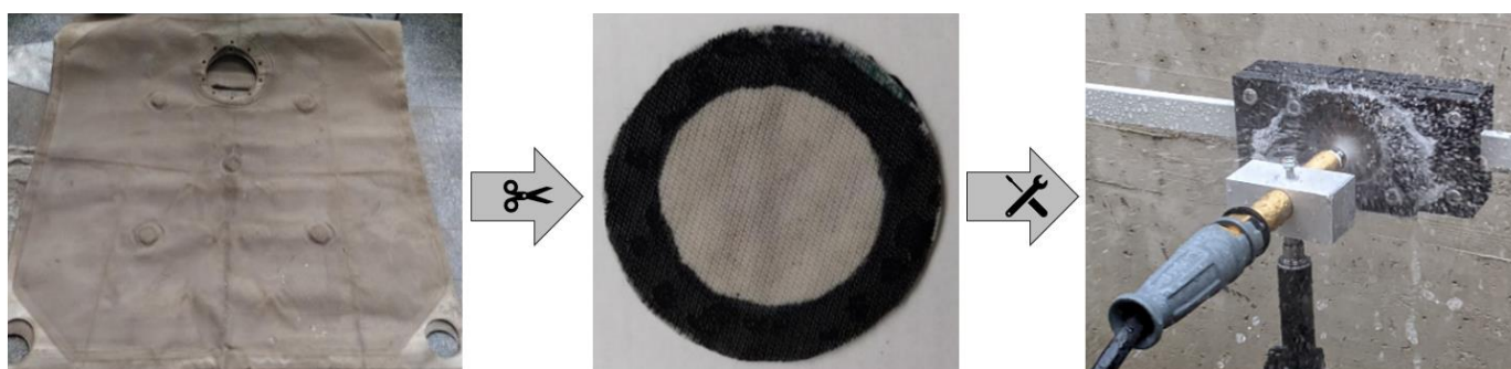
Figure 2. Methodology of permeability test samples preparation including jet cleaning.
