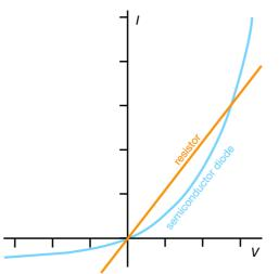
Fig. 4. *I-V* characteristic of a resistor and a semiconductor diode. To characterize the resistor, a single number is sufficient. For the diode a function graph is needed.
