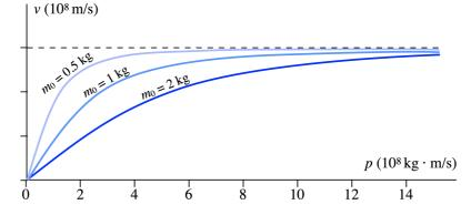
Fig. 2. Dependence of the velocity on the momentum for various rest masses. In all three cases, for increasing momentum, the velocity approaches the same limiting velocity.
