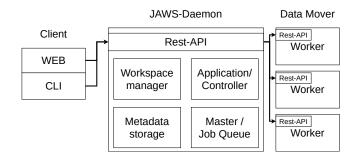
Fig. 2. Design of the JAWS framework. Clients (Web/CLI) access the main daemon via REST API. JAWS Daemon communicates via REST API with distributed worker.
