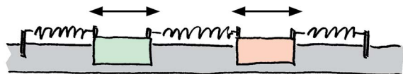
Fig. 3.6 Double oscillator. If only one of the two natural oscillations is excited, both bodies will perform a pure sine movement with equal frequencies. If both natural oscillations are excited at the same time, the position of each of the two bodies will be described by the sum of two sine functions. For each of the two bodies of a double oscillator, the function s(t) is the sum of two sine functions.
