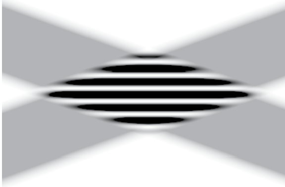
Fig. 4.36 Similar to Fig. 4.35, but the temporal mean value of the y square is displayed here. We can see the interference in the intersection area of the two waves. Light stripes: extinction; dark stripes: amplification
