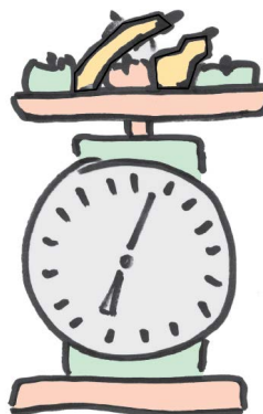
Fig. 6.3 To the question „how heavy are the fruits?“, the scale can give around 200 different answers. The amount of data of an answer is therefore approximately 8 bits.
