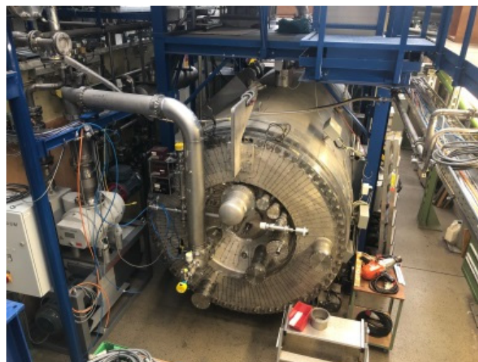
Figure 8. Bird's eye view of the TIMO facility before the main flange insulation for the vessel bake out after air exposure.
