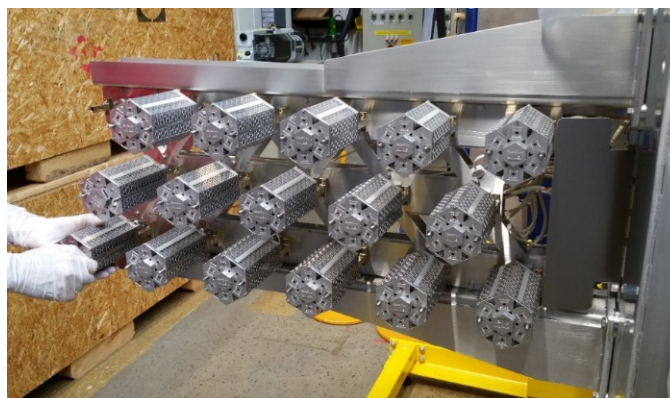
Figure 4. Full NEG pump assembled at the TIMO (test facility for the ITER model pump). The main flange is ready for installation.
