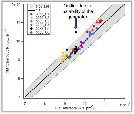
→ Total integrated number concentration within 5% of both reference SMPS (incl. 3081) and reference CPC for well-defined lab aerosol!
