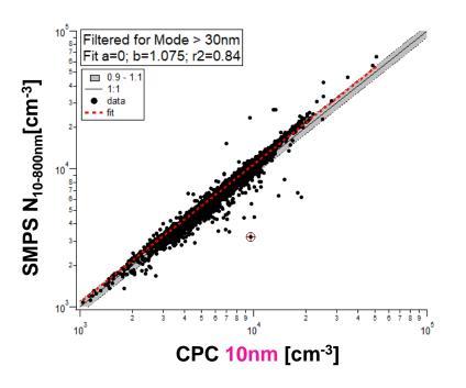
For this analysis SMPS size distribution is not corrected for CPC counting efficiency
