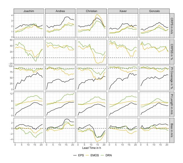
Figure 6.3: Mean CRPS, CRPSS with respect to the raw ensemble predictions, mean PI coverage, mean PI length and mean bias of EMOS, DRN and the raw ensemble predictions as functions of the lead time, averaged over all stations plotted separately for each winter storm within the period from 2011 to 2014.
