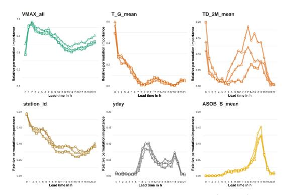
Figure 5.37: Relative permutation importance of selected predictors (Table 5.6) for the three NN-based models dependent on the lead time. Note the different scale of the vertical axes. The abbreviation VMAX\_all refers to the multipass permutation of the features derived from the wind gust ensemble. Different symbols indicate the three model variants ( $\circ$ : DRN,  $\triangle$ : BQN,  $\Box$ : HEN).
