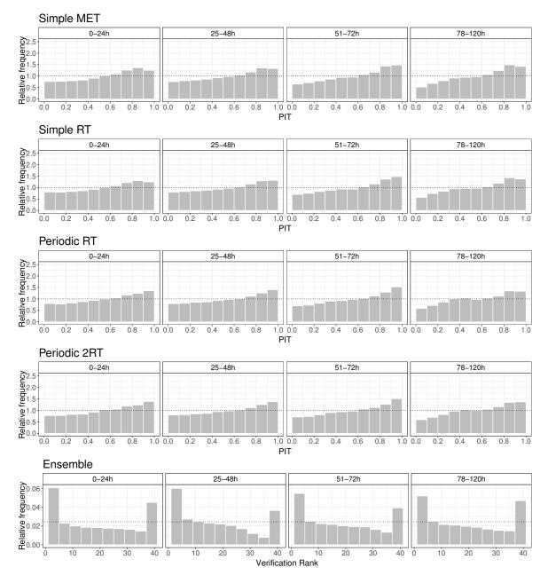
Figure 5.21: PIT histograms of postprocessed and verification rank histograms of raw ensemble forecasts of DNI for the lead times 0–24, 25–48, 51–72 and 78–120 hours for the ICON-EPS dataset.
