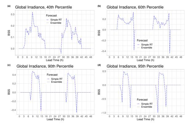
Figure 5.12: BSS of postprocessed forecasts with respect to the raw ensemble as function of lead time for the AROME-EPS dataset, with thresholds corresponding to the 40th, 60th, 90th and 95th percentiles of observed nonzero GHI.
