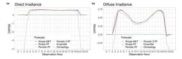
Figure 5.16: CRPSS of postprocessed and raw ensemble forecasts of direct (a) and (b) diffuse irradiance with respect to climatology as functions of the observation hour for the ICON-EPS dataset.
