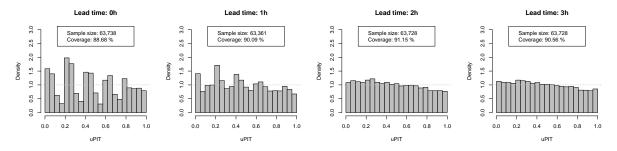
Figure 5.25: PIT histograms of the MBM forecasts for lead times from 0 to 3 hours (left to right) over all stations. Coverage refers to the empirical coverage of a PI with a nominal coverage corresponding to a 20-member ensemble (90.48%).
