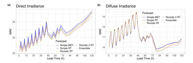
Figure 5.23: MAE of the median forecasts of direct (a) and diffuse (b) irradiance.
