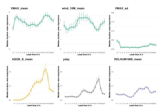
Figure 5.36: Median of stationwise feature importance for selected predictors (Table 5.6) of the QRF model as functions of the lead time. The error bars indicate a bootstrapped 95% confidence interval of the median. Note the different scale of the vertical axes.
