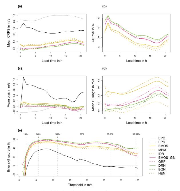
Figure 5.30: Mean CRPS (a), CRPSS with respect to the raw ensemble predictions (b), mean bias (c) and mean PI length (d) of the postprocessing methods as functions of the lead time, averaged over all stations. Panel (e) shows the BSS with respect to the climatological EPC forecast as function of the threshold, averaged over all lead times and stations, where the dashed vertical lines indicate the quantiles of the observed wind gusts at levels given at the top axis.
