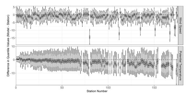
Figure 6.15: Boxplots of the differences in quantile values based on model and station data. Negative values indicate that the value is smaller for the model data.
