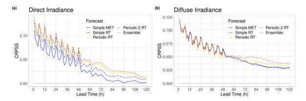
Figure 5.17: CRPSS of postprocessed forecasts of direct (a) and diffuse (b) irradiance with respect to the raw ensemble as functions of the lead time for the ICON-EPS dataset.
