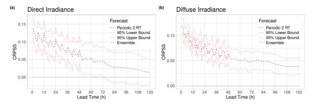
Figure 5.18: CRPSS of the best performing postprocessed forecasts of direct (a) and (b) diffuse irradiance with respect to the raw ensemble together with 95% confidence intervals for the ICON-EPS dataset.
