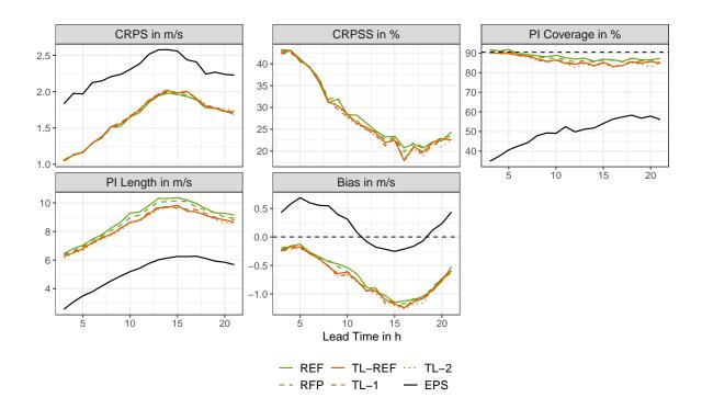
Figure 6.19: Mean CRPS, CRPSS with respect to the raw ensemble predictions, mean PI coverage, mean PI length and mean bias of the feature-based postprocessing approaches as functions of the lead time, averaged over all stations and winter storms.
