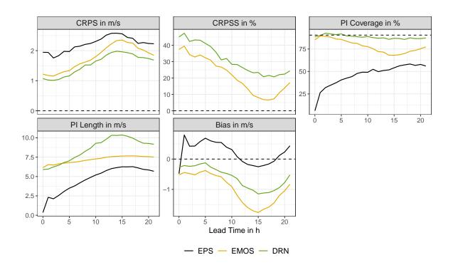
Figure 6.2: Mean CRPS, CRPSS with respect to the raw ensemble predictions, mean PI coverage, mean PI length and mean bias of EMOS and DRN as functions of the lead time, averaged over all winter storms and stations.
