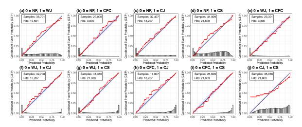
Figure 6.9: CORP reliability diagrams of the conditional RF probabilities comparing two wind features in the all-pairs approach including all 12 storms.
