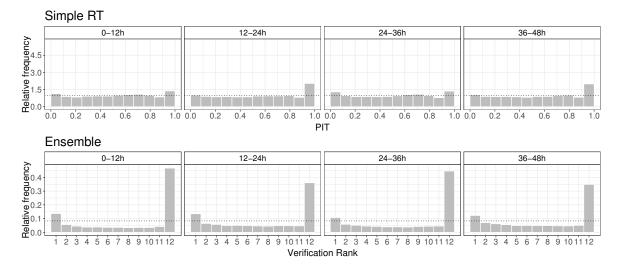
Figure 5.14: PIT histograms of postprocessed and verification rank histograms of raw ensemble forecasts of GHI for the lead times 0–12, 12–24, 24–36 and 36–48 hours.
