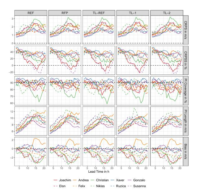
Figure 6.18: Mean CRPS, CRPSS with respect to the raw ensemble predictions, mean PI coverage, mean PI length and mean bias of the feature-based postprocessing approaches as functions of the lead time, averaged over all stations for each winter storm.
