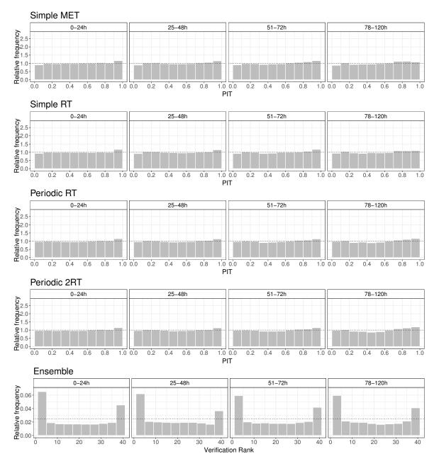
Figure 5.22: PIT histograms of postprocessed and verification rank histograms of raw ensemble forecasts of DHI for the lead times 0–24, 25–48, 51–72 and 78–120 hours for the ICON-EPS dataset.
