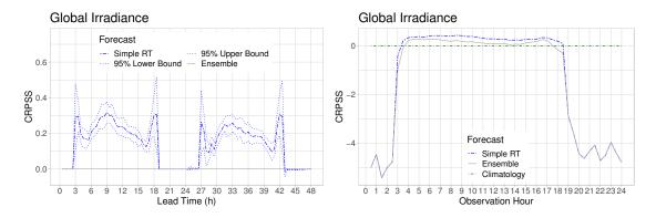
Figure 5.11: CRPSS of EMOS postprocessed forecasts with respect to the raw ensemble together with 95% confidence intervals (left), and CRPSS of postprocessed and raw ensemble forecasts with respect to climatology as functions of the observation hour (right), for the AROME-EPS dataset.
