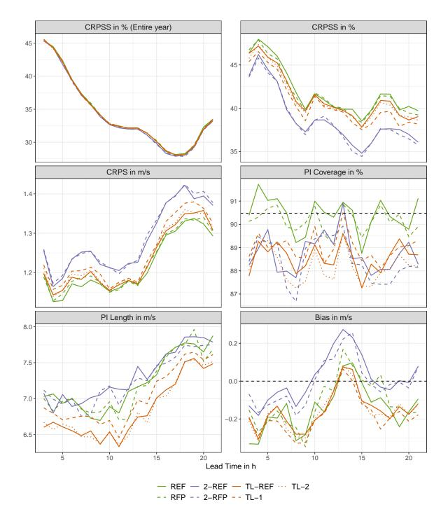
Figure 6.17: CRPSS with respect to the raw ensemble predictions, mean CRPS, mean PI coverage, mean PI length and mean bias of the feature-based postprocessing approaches as functions of the lead time, averaged over all stations for the entire year 2016 (topleft) and for samples that exceed the high-wind threshold (otherwise).
