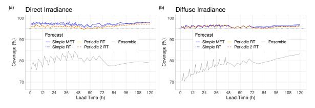
Figure 5.20: Coverage of 95.12% PIs of postprocessed and raw forecasts of direct (a) and diffuse (b) irradiance for the ICON-EPS dataset.
