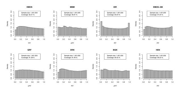
Figure 5.29: PIT histograms of all postprocessing methods, aggregated over all lead times and stations. Coverage refers to the empirical coverage of a PI with a nominal coverage corresponding to a 20-member ensemble (90.48%).
