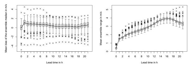
Figure 5.27: Boxplots of the stationwise mean bias of the ensemble median (left) and the mean ensemble range (right) of the COSMO-DE-EPS forecasts as functions of the lead time. The black line indicates the average over all samples.
