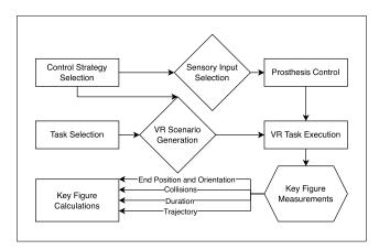
FIGURE 3. Diagram of VR execution flow for each task.
