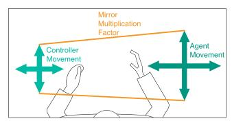
FIGURE 2. Visualization of the mirror multiplication factor.
