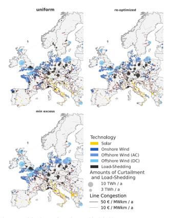
**Fig. 3.** Spatial distribution of curtailment and load-shedding measures across Europe in the highly-resolved operational 1250 node model for the three proposed disaggregation methods after running the operational dispatch. Optimal capacity installations are taken from a model resolution of 97 nodes, and are disaggregated at 1250 regions.
