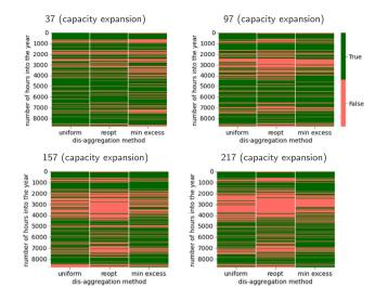
**Fig. 8.** Evaluation if load-shedding measures of the disaggregated highly-resolved operational models occur at times with higher curtailment compared to the low-resolved capacity expansion model, see Eqs. (11)–(12).
