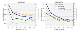
Fig. 2. Amounts of annual load-shedding and curtailment after solving the highlyresolved operational problem with the three proposed disaggregation methods. The number of clusters on the *x*-axis refers to the spatial resolution of the model of which the investment variables are disaggregated at high resolution. Transmission capacity within every cluster is not adjusted. ("regular" setup in Table 2).
