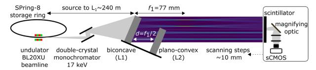
**Figure 6.** The experimental set-up used in this study at the BL20XU beamline, SPring-8, Japan. A monochromatic incoming beam with an energy of 17 keV reaches the gratings located at a position 240 m from the undulator source. The intensities were detected using a CCD camera coupled with a scintillator and magnifying optic. The detector was mounted on a moving stage to measure the wave field along the beam propagation direction.
