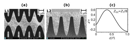
**Figure 5.** Scanning electron microscope (SEM) images of the fabricated biconcave parabolic grating (**a**) and plano-convex parabolic grating (**b**). The comb-shaped support structures in (**a**) were used to minimize the swelling during the electroplating step and were removed when used. Using the micro-lens array profiles observed in (**a**) and (**b**), the  $\xi$  is calculated as a function of  $d/f_1$ , as shown in (**c**).
