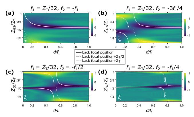
**Figure 3.** Calculated  $\xi$  values corresponding to a binary absorption grating with period equal to that of the parabolic grating, and a duty cycle of 0.5. From (a) to (d),  $f_2$  is set equal to  $mf_2/4$ , ordered by  $m \in \{1, 2, 3, 4\}$ , assuming  $f_1 = Z_T/32$ . The dashed lines indicate the rear focal positions of the L1–L2 lens pair, and solid and dot-dashed lines indicate the positions further downstream from the rear focal position by  $Z_T/2$  and  $Z_T$ , respectively.
