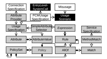
Fig. 4. Simplified access control policy metamodel with PCM integration
