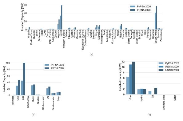
Fig. 8. Total installed generation capacity in Africa by (a) country and (b) technology, including a focus on (c) the installed capacities in Nigeria.
