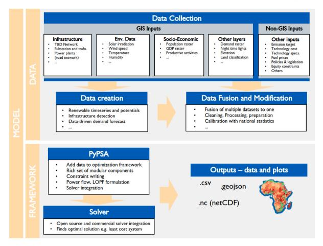
Fig. 1. PyPSA-Earth model design. After providing the configuration parameters and countries of interest, data is collected and processed to be then fed into the PyPSA model framework which enables to perform the desired optimization studies such as least-cost system transition scenarios.
