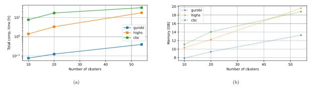
Fig. 9. Solution time (a) and memory requirements (b) for the 2020 Nigeria dispatch optimization for Gurobi 9.5.1, HiGHS 1.2.1 and CBC 2.10.8 solvers at different spatial resolution; solution time is weighted by threads.
