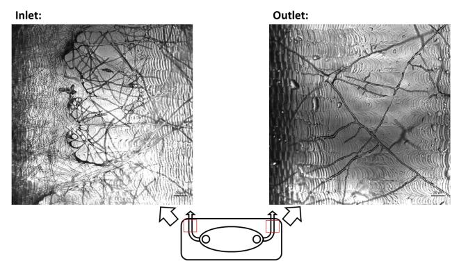
**Fig. 20: Hyphae of** *N. parvum* growing into the inlet and outlet of the MBR system: Brightfield microscopy pictures were taken of both the inlet and outlet of the MBR with an exposure time of 15 ms. An overview schematic of an MBR visualises where the pictures were taken. Hyphae of *N. parvum* grew into both inlet and outlet of the MBR with the density of hyphae being higher in the inlet. The membrane installed into the MBR observed had a pore size of 1  $\mu$ m.
