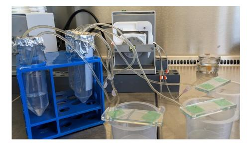
**Fig. 2: Exemplary setup of three singular MBRs:** Three microfluidic bioreactors were installed using a peristaltic pump to create a unidirectional medium flow. The medium runoff of the MBR was fed back into the medium source thus creating a circulating system.
